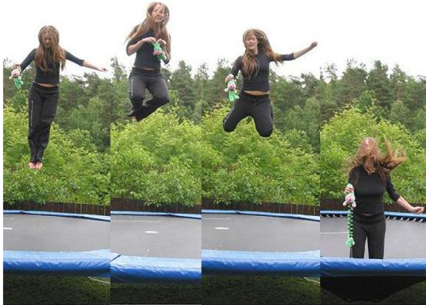
Figure 1. A spiral toy used as an accelerometer during a trampoline jump. Note how the spiral in the toy is contracted while the jumper is in the air, and expanded at the bottom of the jump. Also note how far down the trampoline is displaced in the last photo.
